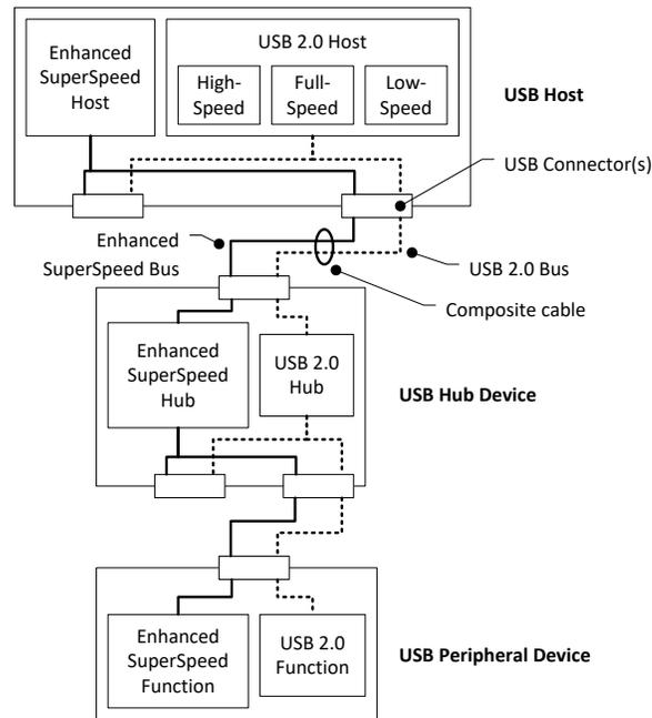
The USB 3.2 interconnect is the manner in which USB 3.2 and USB 2.0 devices connect to and communicate with the USB 3.2 host. The USB 3.2 interconnect inherits core architectural elements from USB 2.0, although several are augmented to accommodate the dual bus architecture.
