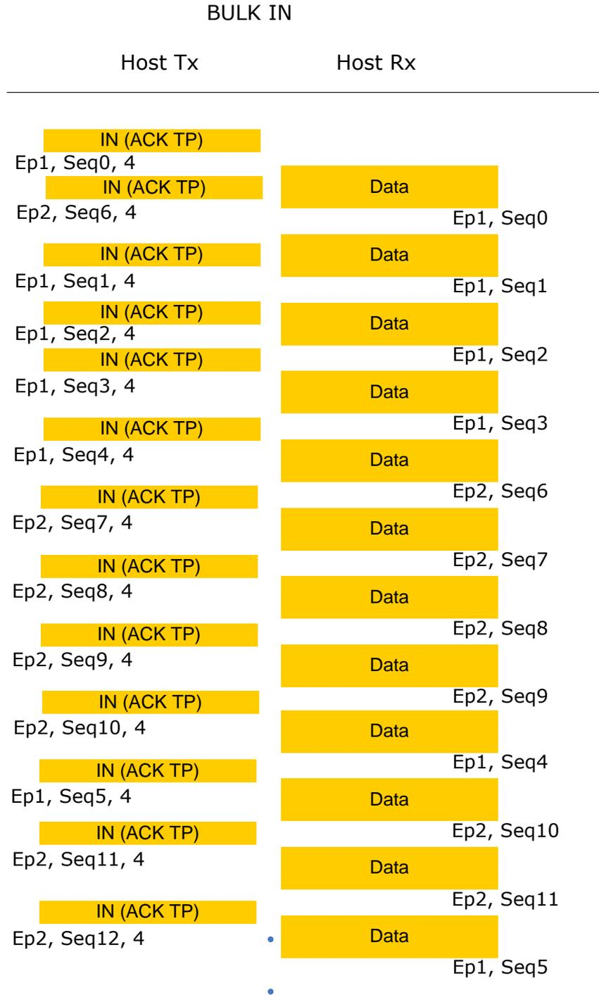
**Figure 8-34. Sample Concurrent BULK and Isochronous IN Transactions**
