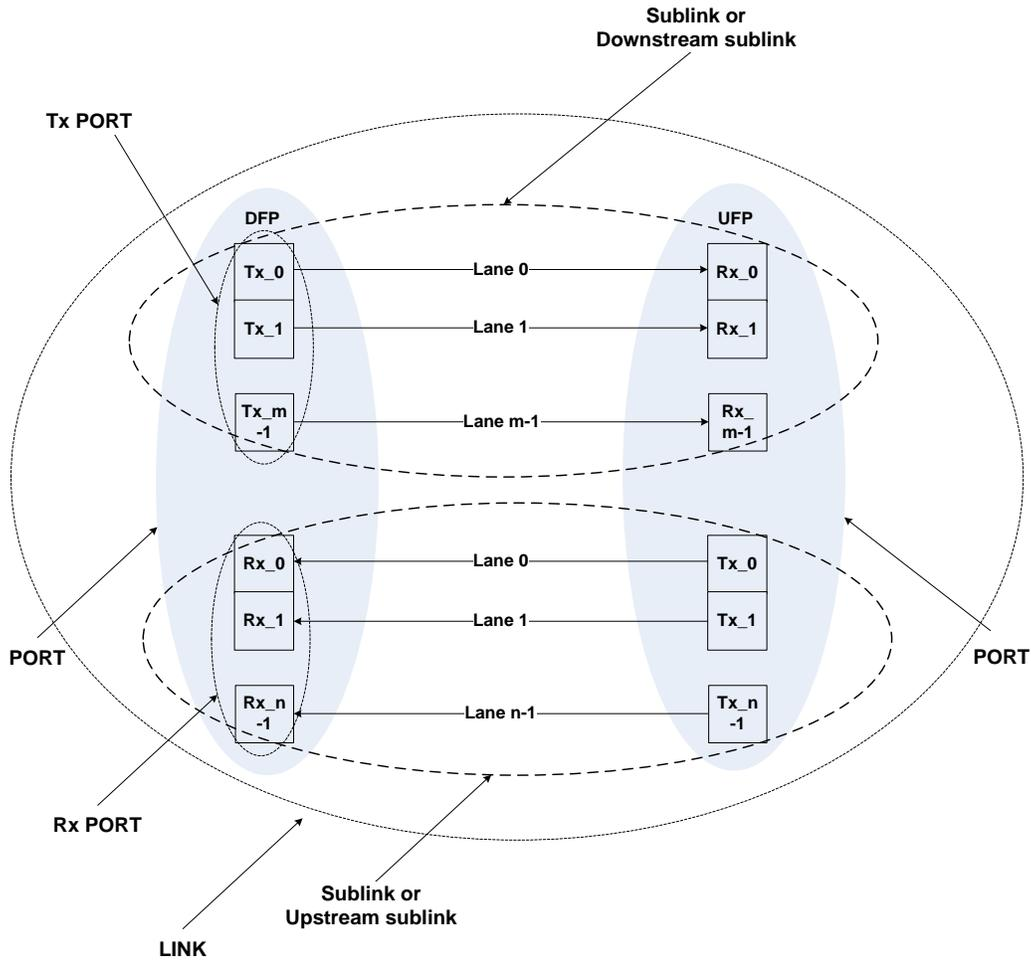
Figure 2-1 illustrates the parts of a port and the connection between ports. The USB 3.1 specification only defines a port with a single Tx and Rx. The inclusion of more than one Rx/Tx pair in a port is for harmonization with the SSIC specification where multiple Rx/Tx pairs are defined. Note: The meanings of the terms used in this figure are not the same as used in PCIe.
