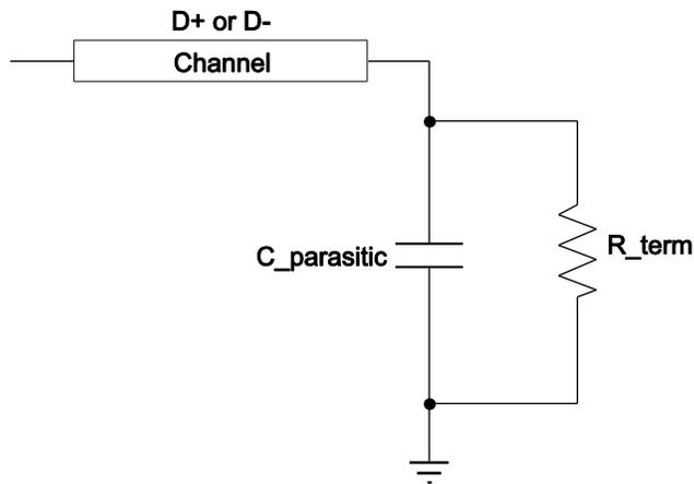
In this circuit, the input buffer is simplified to a termination resistance in parallel with a parasitic capacitor. This simplified circuit is the load impedance.
