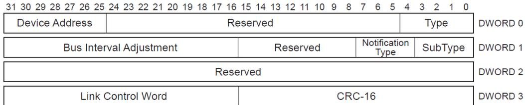
**Table 8-21. Bus Interval Adjustment Message Device Notification**
