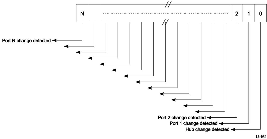
Any time any of the Status Changed bits are non-zero, an ERDY is returned (if an NRDY was previously sent) notifying the host that the Hub and Port Status Change Bitmap has changed. Figure 10-25 shows an example creation mechanism for hub and port change bits.
