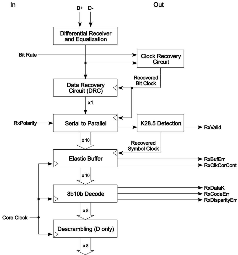
Figure 6-4. Gen 2 Receiver Block Diagram
