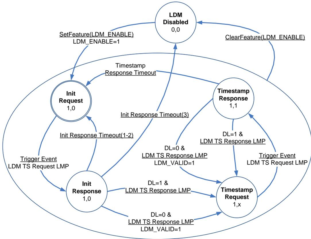
The LDM Requester State Machine shall maintain the following local variable: *Init Response Timeout Counter*.
