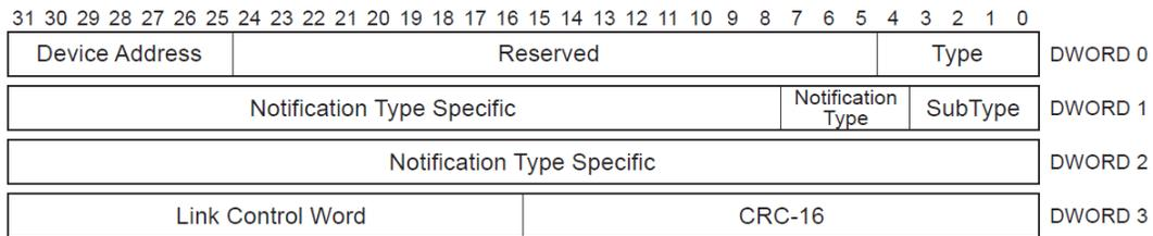
**Table 8-18. Device Notification TP Format (Differences with ACK TP)**
