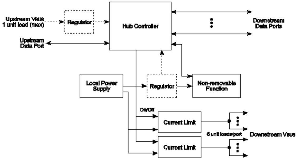
The maximum number of ports that can be supported is limited by the capability of the local VBUS supply.
