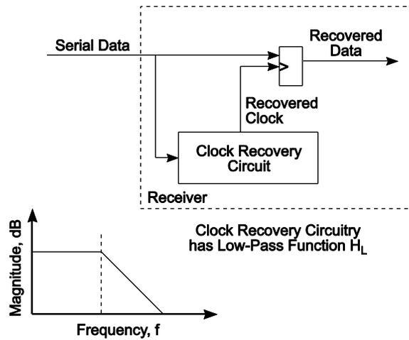
Figure 6-14. “Golden PLL” and Jitter Transfer Functions for Gen 1 Operation
