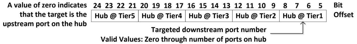
In Figure 8-32, the value in Hub@Tier1 field is the downstream port number of the hub connected directly to one of the root ports on the host to which a second hub is attached and so on.
