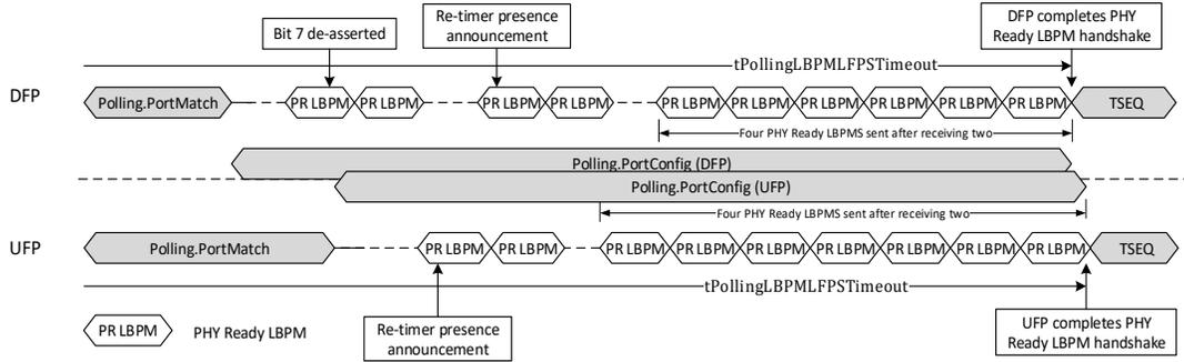
(a) DFP initiates exit to Polling.RxEQ with bit-7 of its PHY Ready LBPM de-asserted. Note that the re-timer presence announcement is also performed during this process. DFP/UFP both continue the  $t_{PollingLBPM LFPSTimeout}$  timer in this substate. DFP/UFP complete the PHY Ready LBPM handshake and transition to Polling.RxEQ.
