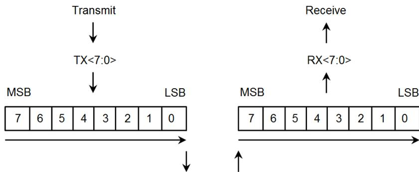
**Figure 6-11. Gen 2 Bit Transmission Order and Framing**
