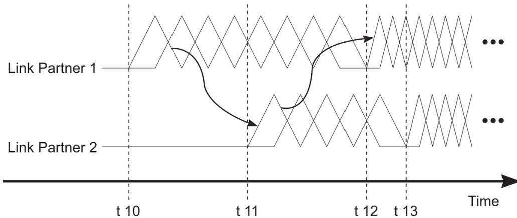
**t<sub>10</sub>** – When Link Partner 1 starts to transmit LFPS, in initiating exit from either U1/U2/U3/Loopback.
