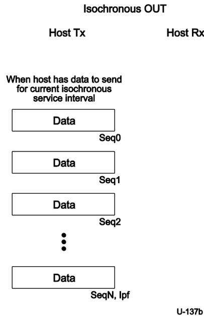
The first DP or ACK TP in each service interval shall start with the sequence number set to 0.
