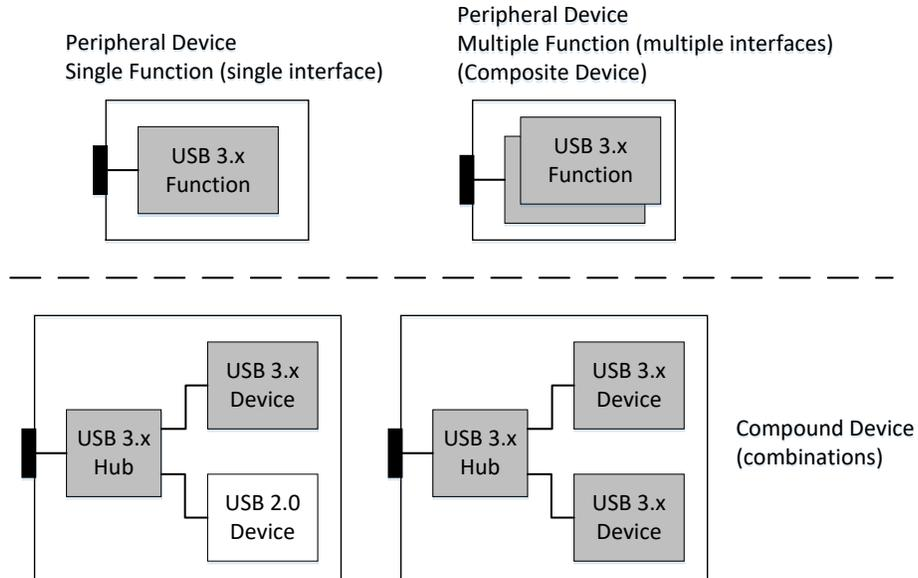
An Enhanced SuperSpeed portion of a peripheral device may only be assembled into one of the following configurations:
