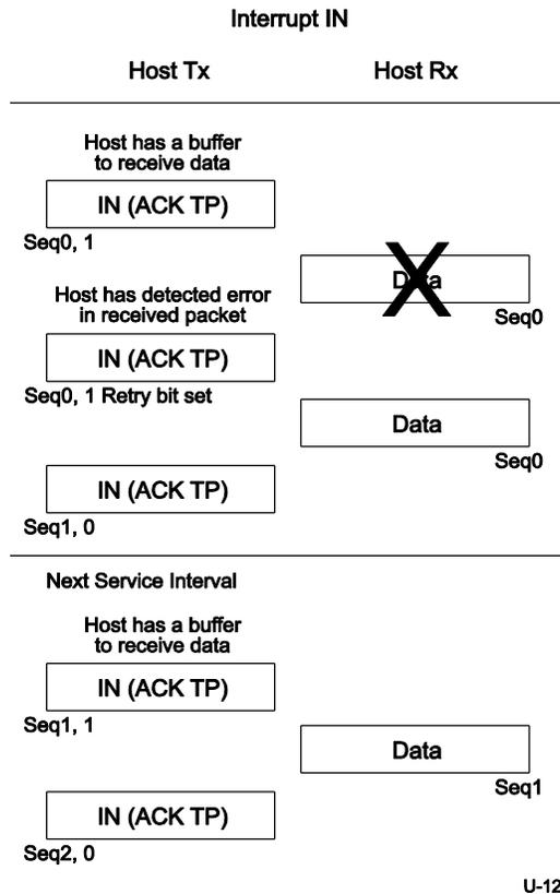
Note: In Figure 8-53 the host retries the data packet received with an error in the same service interval. It is not required to do so and may retry the transaction in the next service interval.
