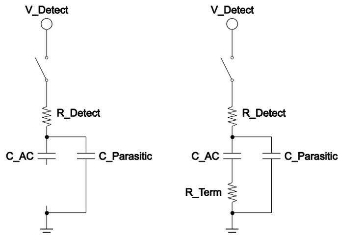
The left side of Figure 6-39 shows the Receiver Detection circuit with no termination present. The right side of the figure is the same circuit with termination.
