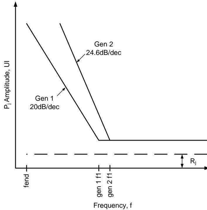
The jitter components used to test the receiver shall meet the requirements of Table 6-28.
