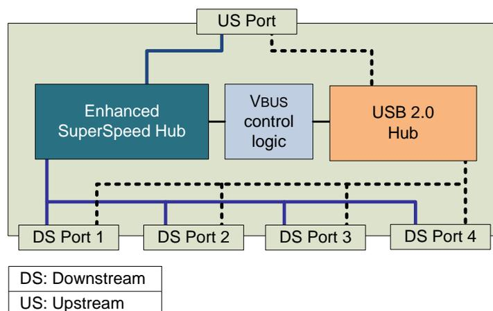
When a USB hub connects on its upstream facing port at Gen 1x1 speed, it shall operate (and be referred to) as a SuperSpeed hub (including operating its downstream ports at no higher than Gen 1x1 speed).
