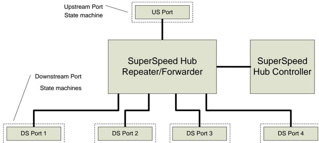
As shown in Figure 10-3, the SuperSpeedPlus hub portion consists of three functional components: the SuperSpeedPlus Upstream Controller, the SuperSpeedPlus Downstream
