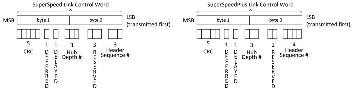
CRC-5 protects the data integrity of the Link Control Word. The implementation of CRC-5 is defined below:
