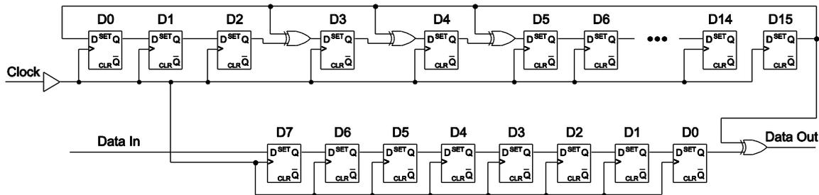
For Gen 1x2 operation, both lanes use the LFSR in Figure 6-9. Details of scrambling for Gen 1x2 mode are contained in Section 6.13.5.
