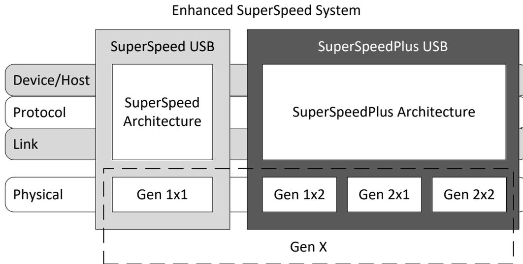
The Enhanced SuperSpeed bus is a layered communications architecture that is comprised of the following elements:
