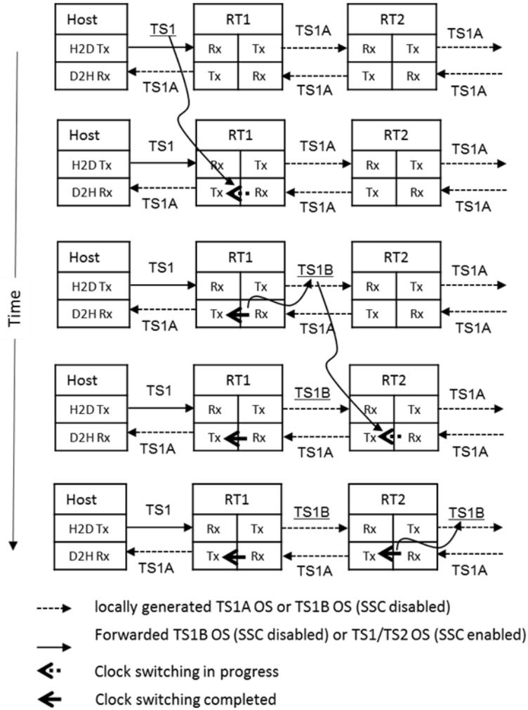
**Figure E-11. Example of Four Bit-Level Re-timer Performing Sequential Clock Switching**
