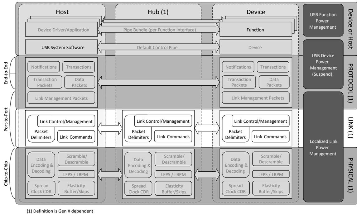
The link layer also facilitates link training, link testing/debugging, and link power management. This is accomplished by the introduction of Link Training Status State Machine (LTSSM).
