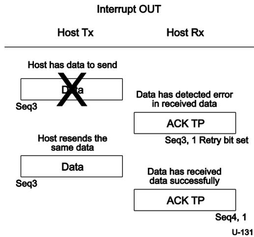
Note: In Figure 8-57 the host retries the data packet received with an error in the same service interval. It is not required to do so and may retry the transaction in the next service interval.
