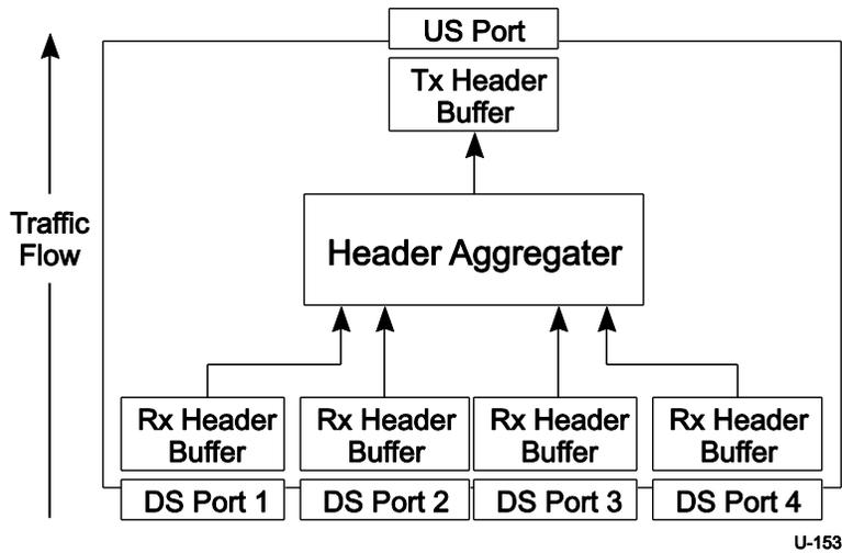
The following lists functional requirements for a SuperSpeed hub buffer architecture with the assumption in each case that only the indicated port on the hub is receiving or transmitting header packets:
