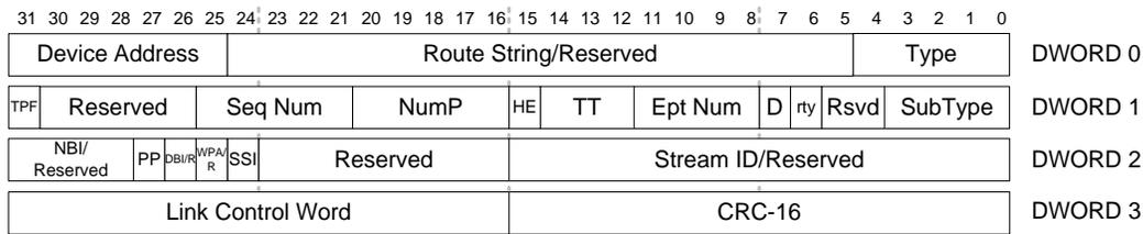
Data Packets include additional information in the header that describes the data block. The Data Block is always followed by a 4-byte CRC-32 used to determine the correctness of the data. The Data Block and the CRC-32 together are referred to as the Data Packet Payload.
